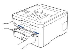
4. Using both hands, place one sheet of paper in the manual feed slot until the front edge touches the paper feed roller. When you feel the machine pull it in, let go.
