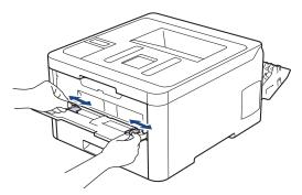
4. Using both hands, place one sheet of paper in the manual feed slot until the front edge touches the paper feed roller. When you feel the machine pull it in, let go.
