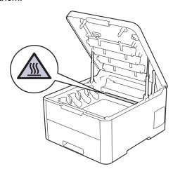
2. Remove the toner cartridge and drum unit assemblies.
