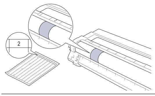
11. Wipe the surface of the drum gently with a dry cotton swab until the mark on the surface comes off.
