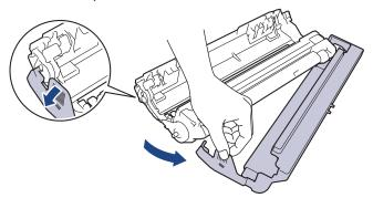
7. Reinsert the toner cartridge firmly into the new drum unit until you hear it lock into place.
