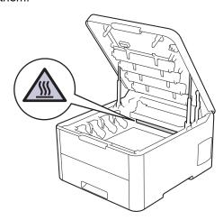
3. Remove the toner cartridge and drum unit assembly for the colour shown on the LCD.
