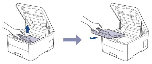
5. Unpack the new belt unit and insert it into the machine.
