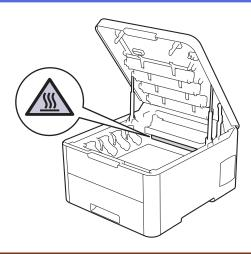
7. The colour of printed dots on the Drum Dot Check Sheet is the colour of the drum you should clean. Remove the toner cartridge and drum unit assembly that matches the colour causing the problem.
