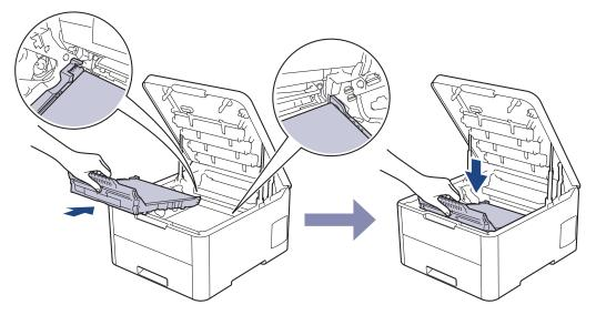
9. Reinsert each toner cartridge and drum unit assembly into the machine. Make sure that you match the toner cartridge colour to the same colour label on the machine for all four toner cartridge and drum unit assemblies.
