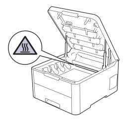
3. Remove all of the toner cartridge and drum unit assemblies.
