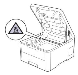
3. Remove all of the toner cartridge and drum unit assemblies.
