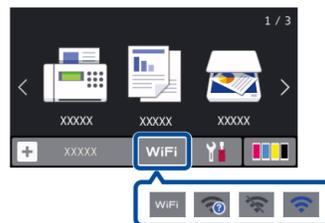
Even if you do not have a wireless access point/router, you can connect your device and your machine directly. For additional wireless network support, go to [support.brother.com/wireless-support](http://support.brother.com/wireless-support).
