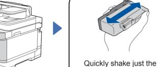
black ink cartridge horizontally 15 times as shown, before inserting it into the machine.
