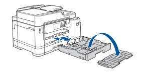
Pull the paper tray completely out of the machine as shown by the arrow. Take off the tray top cover.
