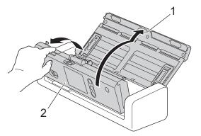
3. In the document feeder unit, clean the glass strips (1) (2) with a soft lint-free cloth moistened with water.
