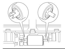
6. Slide the Pick Up Roller(1) to the left edge while turning the Pick Up Roller.
