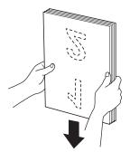
4. Position the pages so that the leading edges are aligned at a slight angle in the feed direction.
