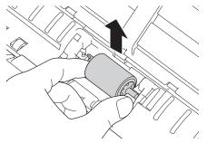
5. Place a new Pick Up Roller into the machine.
