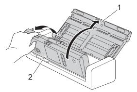
3. Wipe off the paper dust accumulated on the Document Scanning Position Sensor (1) with a soft lint-free cloth moistened with water.
