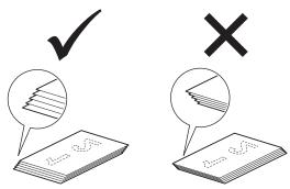
5. Slide the Feed Selector to the left and confirm that it is in ADF Mode. Place your document, *face down, top edge first* in the ADF between the Paper Guides until you feel it touch the inside of the machine. Feed thin pages slowly and carefully to keep the edge from folding.
