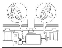
9. Slide the Pick Up Roller(1) to the left edge while turning the Pick Up Roller.
