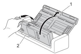
2. Pinch the Pick Up Roller Cover (1) and then pull the cover up and remove.
