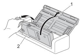
2. Pinch and pull the Separation Pad upwards.
