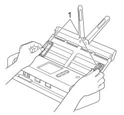
2. Slide the Feed Selector to the left and confirm that it is in ADF Mode. Place your document, *face down, top edge first* in the ADF between the Paper Guides until you feel it touch the inside of the machine. Feed thin pages slowly and carefully to keep the edge from folding.
