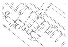
4. Wipe off the paper dust accumulated on the Card Sensor (1) with a soft lint-free cloth moistened with water.
