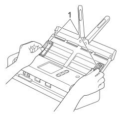
2. Slide the Feed Selector to the left and confirm that it is in ADF Mode. Place the card, *face down, top edge first* in the ADF between the Paper Guides until you feel it touch the inside of the machine.
