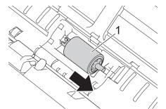
4. Pinch and pull the Pick Up Roller out of the machine.
