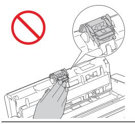
4. Pinch the Pick Up Roller Cover (1) and then pull the cover up and remove.
