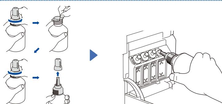
Remove the film and tighten the cap firmly.
