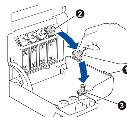
Open the ink tank cover ①, remove the cap ②, and place it on the back of the cover ③.
