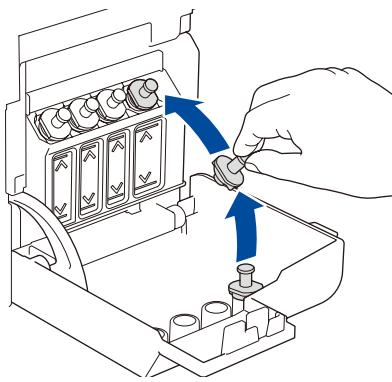
Replace the ink tank cap. Repeat step 5 for the other ink tanks, and then close the ink tank cover.
