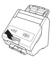
3 Lift the lower part of the Foil Holder and Cartridge Assembly ①, and then lift the entire Foil Holder and Cartridge Assembly upwards ② to remove it from the machine.
