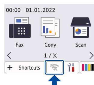
Select the SSID (Network Name) for your access point/router and enter the Network Key (Password). When the wireless setup is successful, the LCD displays [Connected].
