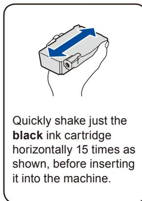
Quickly shake just the **black** ink cartridge horizontally 15 times as shown, before inserting it into the machine.
