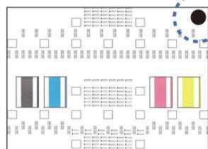
Follow the LCD instructions to print the Adjustment Sheet. The black circle mark is located in the upper right corner of the sheet.
