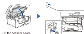
Connect the telephone line cord. Use the socket marked **LINE** and guide the cord out the back of the machine.
