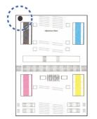
Follow the LCD instructions to print the Adjustment Sheet. The black circle mark is located in the upper left corner of the sheet.
