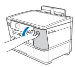
3 Quickly shake just the <u>black</u> ink cartridge horizontally 15 times as shown, before inserting it into the machine. The other inks do not need to be shaken.
