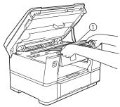
13 Move the print head, and then remove any material remaining in this area. Make sure pieces of material are not left in the corners of the machine (①) and (②).
