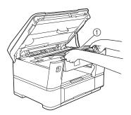
11 Move the print head, and then remove any material remaining in this area. Make sure pieces of material are not left in the corners of the machine (①) and (②).
