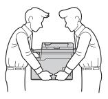
If you use a Lower Tray, DO NOT carry the product with the Lower Tray, as you may be injured or cause damage to the product because it is not attached to the Lower Tray.
