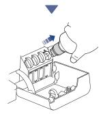
When finished, remove the bottle, pulling the nozzle slowly so the ink does not spill.
