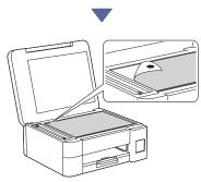
Place the Adjustment Sheet face down on the scanner glass, making sure the black circle is in the upper left corner of the scanner glass, as shown.
