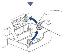
Remove the cap from inside the ink tank cover and seal the ink tank.
