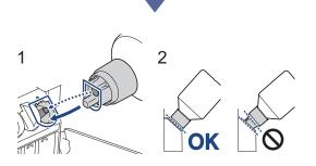
Align the bottle so that the pin on the ink tank can be inserted into the hole in the bottle, as shown in (1).
