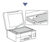
Place the Adjustment Sheet face down on the scanner glass, making sure the black circle is in the upper left corner of the scanner glass, as shown.
