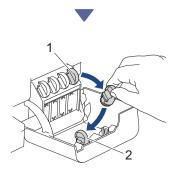
Remove the cap (1) and place it inside the back of the cover (2).
