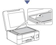
Place the Adjustment Sheet face down on the scanner glass, making sure the black circle is in the upper left corner of the scanner glass, as shown.
