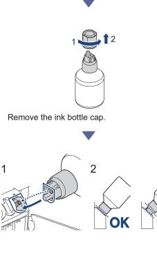
Align the bottle so that the pin on the ink tank can be inserted into the hole in the bottle, as shown in (1).
