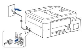
Insert the telephone line cord into the socket marked **LINE**.
