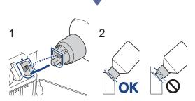
Align the bottle so that the pin on the ink tank can be inserted into the hole in the bottle, as shown in (1). Slide the bottle onto the pin at the angle shown in (2) until the cap is flush with the ink tank surface. (You will hear a click when you insert it for the first time.)
