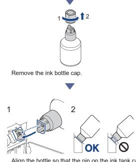
Align the bottle so that the pin on the ink tank can be inserted into the hole in the bottle, as shown in (1).
