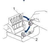
Remove the cap (1) and place it inside the back of the cover (2).
