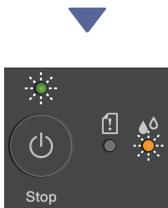
During the initial cleaning, both the Power and Ink LEDs will flash.
