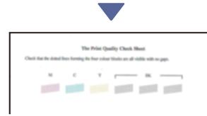
When the initial ink system cleaning has finished, the machine prints the Print Quality Check Sheet.
