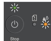
When the Power LED starts flashing slowly, press and hold the **Mono Copy** button for three seconds.
