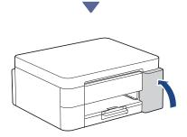
After installing all of the four ink cartridges, close the ink cartridge cover.
