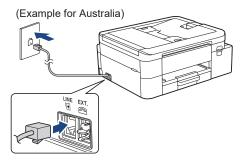
Insert the telephone line cord into the socket marked LINE.
