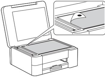
Place the Adjustment Sheet face down on the scanner glass, making sure the black circle is in the top left corner of the scanner glass, as shown.
