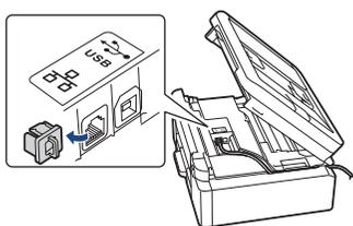
For USB connection or wired network connection (certain models only), locate the correct port (based on the cable you are using) inside the machine, as shown.
