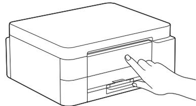
Check the LCD messages to continue the setup. When the ink preparation message appears, follow the LCD instructions to perform the initial ink system cleaning. Cleaning can take a few minutes, and you can perform the next step during this time.
