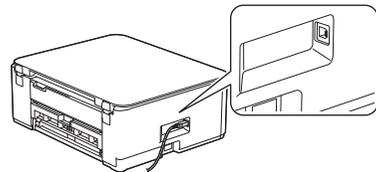
For USB connection, locate the correct port on the side of the machine, as shown.
