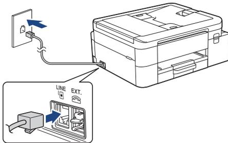
Insert the telephone line cord into the socket marked **LINE**.
