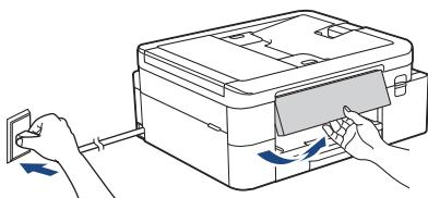
The machine powers on automatically.
