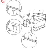
When carrying the product, remove the trays if they have been extended to hold large paper. The weight of the paper could cause the trays to fall and cause injury to you or others
