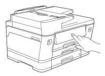
When the initial ink system cleaning has finished, print the Print Quality Check Sheet: Press [Start].
