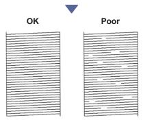
On the machine's LCD, select the images that closely match the image for each colour on the Print Quality Check Sheet, and then restart the cleaning procedure, if required.
