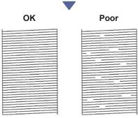
On the machine's LCD, select the images that closely match the image for each colour on the Print Quality Check Sheet, and then restart the cleaning procedure, if required.
