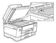
Place the Adjustment Sheet face down on the scanner glass, making sure the black circle is in the top left corner of the scanner glass, as shown.
