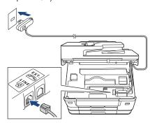
Insert the telephone line cord into the socket marked LINE and guide the cord out of the back of the machine.
