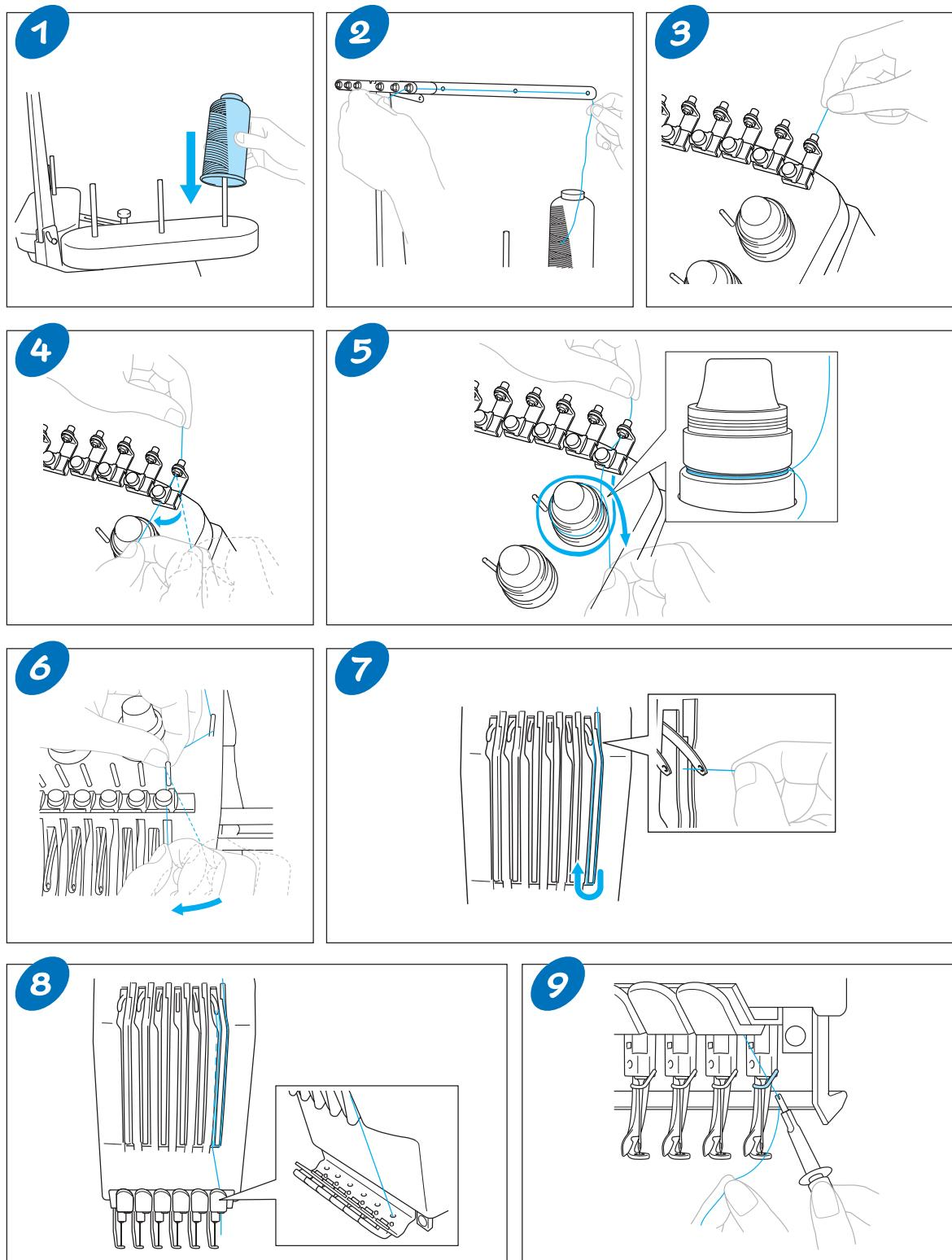
◆ Threading the needle
