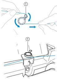
① Thread guide for bobbin winding
