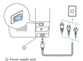
Press the right side of the main power switch on the right side of the machine (set it to "|").
