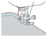
When sewing along a curve while using a zigzag stitch, select a shorter stitch length in order to obtain a finer stitch.
