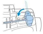
Place the upper thread spool for the needle on the right side onto the extra spool pin, and then secure it with the spool cap.
