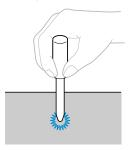
• When using the eyelet punch, place thick paper or some other protective sheet under the fabric before punching the hole in the fabric.
