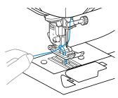
Pull out about 5 cm (2 inch) of the bobbin thread under the presser foot toward the rear of the machine.
