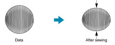
Note: When using Satin stitch in a wide area, the needle may move out of position by about 10 mm with some machines. To avoid this, use the above mentioned alternate method.
