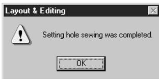
When a pair of patterns are set to hole sewing, they cannot be moved separately. If you need to readjust their relative position, you must first select the circle or the broken line with the selection cursor
