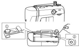
Bobbin-winding tension disc
