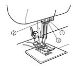
Right needle thread passes through thread guide
