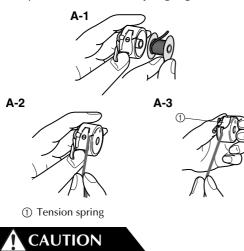
• Make sure you set the bobbin so the thread unrolls in the correct direction. If the thread unrolls in the wrong direction, it may cause the thread tension to be incorrect or break the needle.
