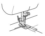
• You can use reverse sewing for locking the end of seams and where you need to strengthen a stitch.
