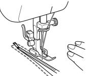
**6** To sew the opposite side of the zipper, release the foot by raising the lever located at the back of the presser foot, position the zipper foot on the other side of the zipper and continue sewing using the notch on the other side.
