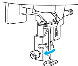
**9 Firmly tighten the presser foot holder screw.**
