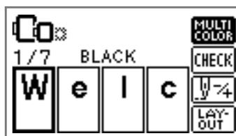
The needle progresses one color or one stitch (if pressed continuously, 9 stitches to 20 stitches) at a time and changes the position for starting the embroidery. This is used when a specific color is not sewn or when restarting the sewing machine after power has been turned off in the middle of the operation.
