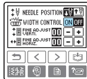
▶ The machine is now set so that the stitch width can be controlled with the sewing speed controller.
