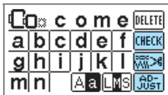
**CHECK** When a specific pattern is selected, press this key and then, press to switch the display. The sewing settings such as the specified alphabet character string and color are confirmed.
