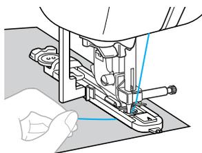
▶ Once sewing is completed, the machine automatically sews reinforcement stitches, then stops.
