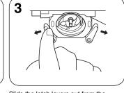
Raise the needle to its highest position, Slide the latch levers out from the retaining ring.
