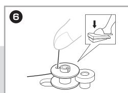
While holding the end of the thread, gently depress the foot controller. 拉著縫紉線末端,並輕輕蹅下腳掣。
