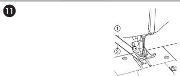
Pass the upper thread ① through the presser foot, and then pull out about 10 cm (4") of the upper thread ① and the lower thread ② toward the rear of the machine. 把上線①繞過壓靴,然後從後方②拉出大約10厘米(4吋)的縫紉線。
