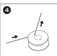
Pass the thread through the hole on the bobbin from the
