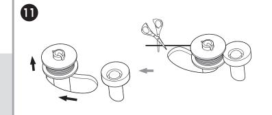
Cut the thread, slide the bobbin winder shaft to the left, and then remove the bobbin.
