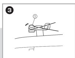
Pass the thread around the bobbin winding tension disk 1.
