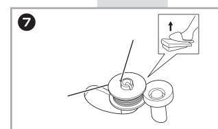
Wind the thread around the bobbin a few times, then take your foot off of the foot controller.
