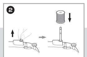
Pull up the spool pin and place a spool of thread on this pin.
