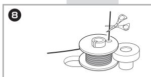
Trim the excess thread above the bobbin. 把線芯上多餘的縫紉線剪斷
