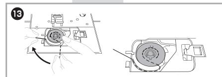
Insert the bobbin into the shuttle, pass the thread through the slot.
