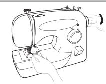
While holding the end of the upper thread, slowly turn the balance wheel toward you once to lower, then raise the needle.
