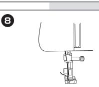
Thread the needle from front to back. 由前向後方向穿線。
