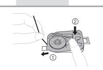
While pulling the thread to the left of the needle plate, move the bobbin cover to its original position.
