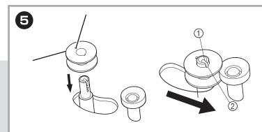
Align the spring ① with the groove ② and place the bobbin onto the bobbin winder shaft, and then slide the bobbin winder shaft to the right. 較準彈簧①於槽位②上,並將線芯置入繞線卷軸器內,再把卷 軸器推向右方。
