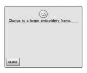
This message is displayed when the machine is in embroidery mode and the small frame is attached, and the selected pattern does not fit in the small frame.
