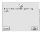
This message is displayed when the machine has recognized the embroidery position mark. Remove the embroidery positioning
