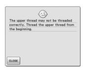
This message is displayed when it seems that the upper thread has not been threaded correctly.
