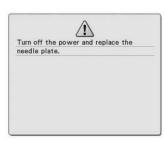
This message is displayed when you try to sew with a stitch other than a middle needle position stitch while the single-hole needle plate is installed.
