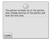
This message appears when the built-in camera is being used to align the embroidery position, but the embroidery positioning sticker is too near an edge or the pattern extends from the embroidery frame. Change the positioning of the embroidery position sticker, and then try aligning the position again. See page 208.
