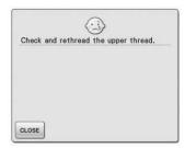
This message is displayed when the upper thread is broken or not threaded correctly, and the "Start/Stop" button or the "Reverse/ Reinforcement Stitch" button is pressed.
