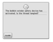
This message is displayed when the bobbin is being wound, and the motor locks because the thread is tangled, etc.
