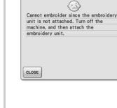
This message is displayed when the "Start/Stop" button is pushed and the machine is in embroidery mode, but the embroidery unit is not attached.
