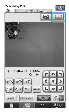
Press the positioning keys to move the embroidery frame until the thread mark on the fabric is aligned on the starting point in the camera view window.
