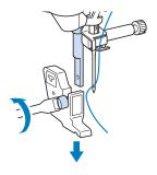
Set the operation lever of the walking foot so that the needle clamp screw is set between the fork. Position the shank of the walking foot on the presser foot bar.
