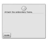
This message is displayed when the machine is ready to sew an embroidery pattern, and the "Start/Stop" button is pushed while the embroidery frame is not attached.
