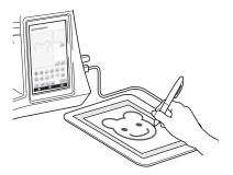
The included pen tablet can be used to perform My Custom Design operations effectively, along with normal screen operations. Since the range of operation with the pen tablet is wider than the machine's LCD screen, you can easily perform intricate procedures.
