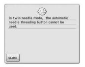
This message is displayed when the automatic needle threading button is pushed while twin needle sewing is
