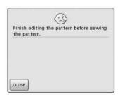
This message is displayed when the "Start/ Stop" button is pushed while the machine is in embroidery edit mode and a pattern is being edited.
