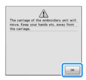
→ After the thread is automatically cut, the carriage will move.
