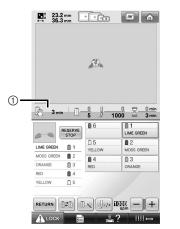
① Time until the machine stops
