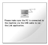
Machine failed to communicate with the PC in the Link mode. Turn the machine off, and then turn the machine on again.
