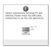
Machine cannot receive any data from the PC in the Link mode. Turn off the machine, and check the USB connection. After connecting the USB cord securely, turn on the machine again.
