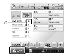
The needle bar number changes and appears to indicate the selected needle bar.
