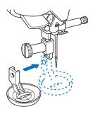
6 Tighten the screw with the included screwdriver.
