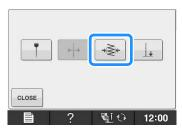
→ The stitching width setting screen appears, and the guideline marker flashes at the present left side of the stitch width.
