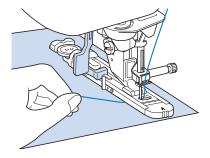
Once sewing is completed, the machine automatically sews reinforcement stitches, and then stops.
