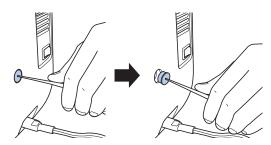
Firmly insert the sensor pen holder into the hole where the protective cap was removed.
