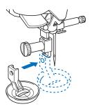
Tighten the screw with the included screwdriver.
