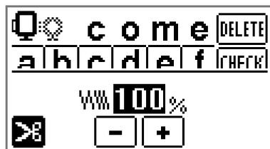
**MM>B** Press this key to select or cancel programmed thread cutting. When programmed thread cutting is set, the thread is cut automatically after reinforcement.
