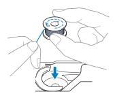
If the bobbin is inserted with the thread unwinding in the wrong direction, sewing will be done with an incorrect thread tension.
