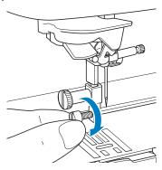
Set the operation lever of the walking foot so that the needle clamp screw is set between the forks. Position the shank of the walking foot on the adapter attached to the presser foot bar.
