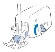
When the feed position lever is down, the black roller belt on the dual feed is engaged.
