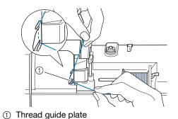
While holding the thread in your right hand, pass the thread through the thread guide in the direction indicated.
