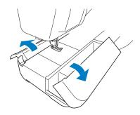
A presser foot storage tray is stored in the accessory compartment of the flat bed attachment.
