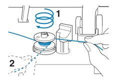
Pass the end of the thread through the guide slit in the bobbin winder seat, and pull the thread to the right to cut the thread with the cutter.
