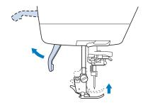
Push the black button on the presser foot holder and remove the presser foot.
