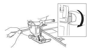
→ A loop of the bobbin thread comes out through the hole in the fabric.
