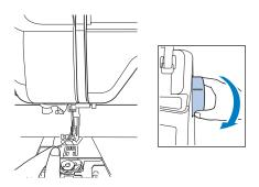
Gently pull the upper thread to bring the bobbin thread up through the needle plate.
