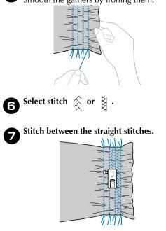
Pull out the threads for the straight stitches.
