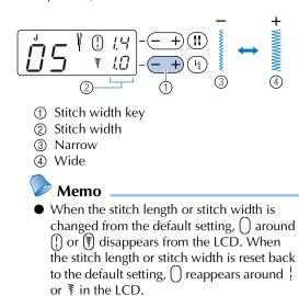
If the stitch width of the selected stitch cannot be adjusted, "--" appears to the right of ₹ in the LCD.
