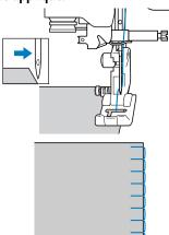
• When sewing around corners, stop the machine with the needle in the fabric just outside of the appliqué, raise the presser foot lever, and then turn the fabric as needed to change the sewing direction.
