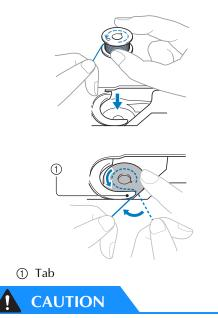
Be sure to hold down the bobbin with your finger and install the bobbin so that the thread unwinds in the correct direction. otherwise the needle may break or the thread tension will be incorrect.
