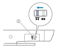
① Feed dog position switch (as seen from the rear of the machine)
