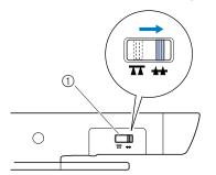
Drop feed lever (as seen from the rear of the machine)
