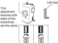
Turn the buttonhole fine-adjustment screw with a large screwdriver as indicated in the illustrations, according to the buttonhole appearance.
