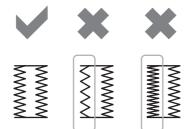
If the left side is too open or tight compared with the right side, adjust the buttonhole fine-adjustment screw
