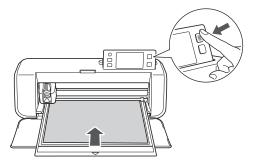
The mat is fed in to complete the preparations for cutting.
