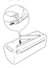
Dampen a soft lint-free cloth with water and firmly wring it out, and then wipe the scanner glass at the inside on the bottom of the machine.
