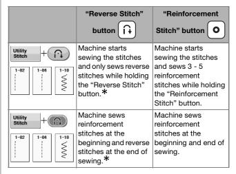
\* If "Reinforcement Priority" on the settings screen is set to "ON", reinforcement stitches are sewn instead of reverse stitches.
