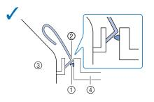
Notch (1) does not fit firmly under the bend in the lever (2).
