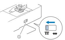
① Feed dog position switch (as seen from the rear of the machine)
