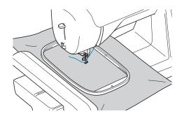
**5** Trim the excess thread at the end of the seam. If the end of the seam is under the presser foot, raise the presser foot, then trim the excess thread.
