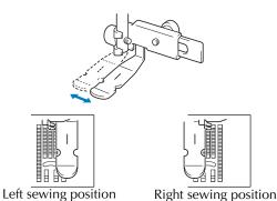
6 Change the needle position so that the needle does not touch the presser foot.
