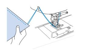
When the needle has stopped moving, raise the presser foot and remove the fabric.
