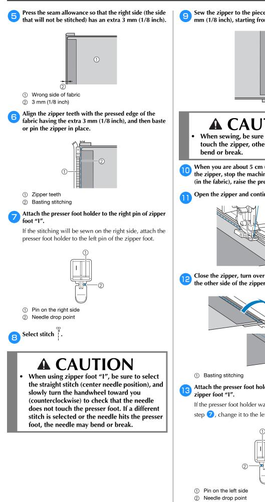
Sew the zipper to the piece of fabric with the extra 3 mm (1/8 inch), starting from the base of the zipper.
