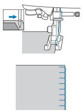
When sewing around corners, stop the machine with the needle in the fabric just outside of the appliqué, raise the presser foot lever, and then turn the fabric as needed to change the sewing direction.
