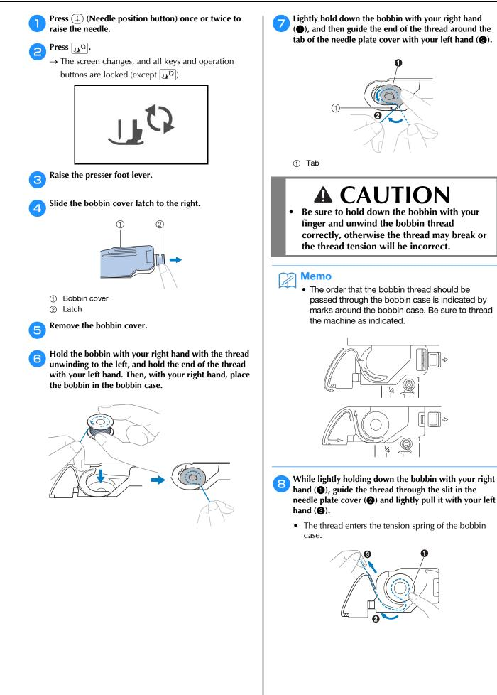
While lightly holding down the bobbin with your right hand (①), continue guiding the thread through the slit with your left hand (②). Then, cut the thread with the cutter (③).
