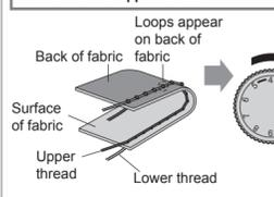
**Solution:** Increase the tension by turning the upper tension control dial to a higher number.
