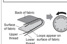
**Solution:** Reduce the tension by turning the upper tension control dial to a lower number.
