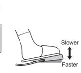
Press the foot controller down to start sewing. Take your foot off the foot controller to stop sewing.
