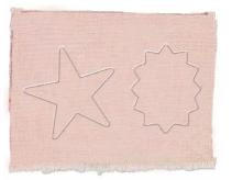
The blade scale setting is insufficient. Adjust the setting on the holder scale.
