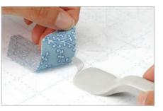
Do not remove the sheet excess. If an uneven surface is created, the fabric may not be cut cleanly.
