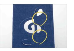
In order to cut cleanly, a mat with an adequate adhesive strength as well as appropriate blade scale and cut pressure settings are required. Replace the standard mat with a new one, and adjust the settings.
