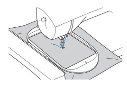
Trim the excess thread at the end of the seam. If the end of the seam is under the presser foot, raise the presser foot, then trim the excess thread.
