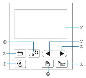
1 LCD (liquid crystal display) (touch panel) Selected pattern settings and messages are displayed. Touch the keys displayed on the LCD to perform operations. For details, refer to "LCD Operation" on page B-9.
