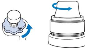
Loosen by turning counterclockwise.
