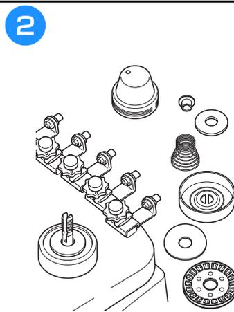
Remove any lint and dust from the two pieces of felt washers (top, bottom) inside the tension dial.
