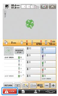
→ After the outlines of the cutout areas are sewn, the areas will be cut with the cutwork needles. After cutting with the cutwork needles, the machine will stop.
