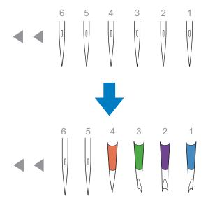
When using the cutwork needles, the fabric will be cut.
