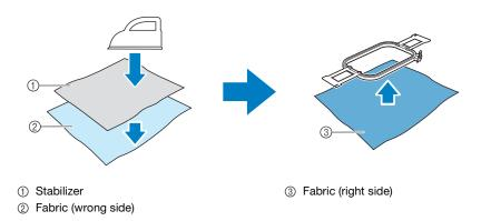
When using fabric that cannot be ironed, such as organza, place water-soluble stabilizer above and below the fabric, and secure the sheets with an embroidery frame.
