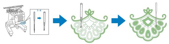
Import a cutwork pattern from the enclosed CD-ROM1 (for machines) to the machine in order to create cutwork.
