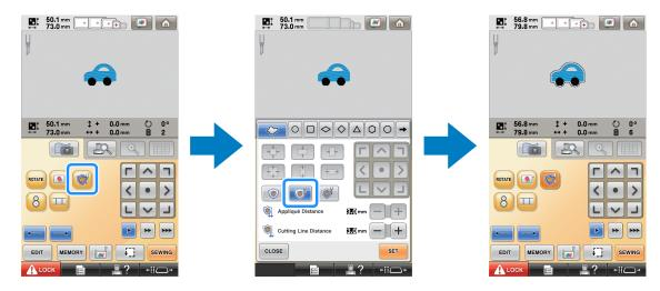
The sections of the design where the cutwork needles will be used are indicated in the embroidering screen as shown below.
