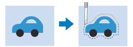
The cutting line for the appliqué piece (APPLIQUE MATERIAL) will also be cut using the cutwork needles.
