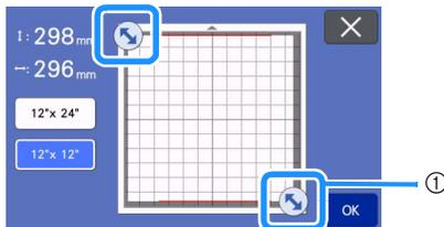
① Area resizing key (Using the touch pen (stylus), touch the key, and then drag it around the screen to specify the area.)
