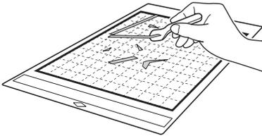
Use tweezers (available either as optional accessories or commercially) to remove any fabric threads attached to the mat.
