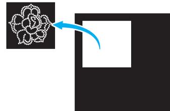
**10** Place the template sheet on a flat surface with the backing down, and then quickly peel the template sheet off horizontally.
