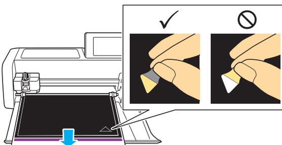
**8** If the trial cutting of the pattern was cut properly, touch the "Start" key and cut the rhinestone pattern.
